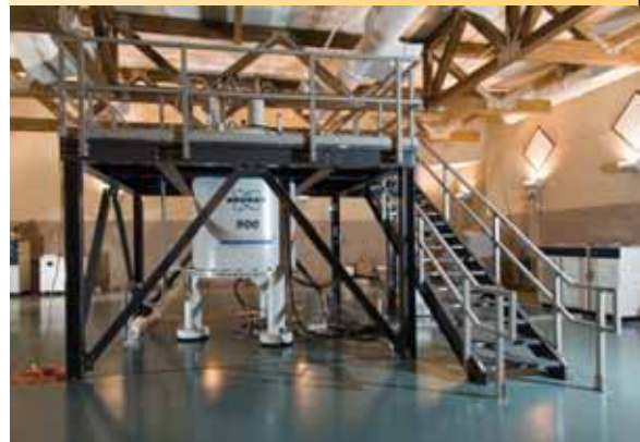
The Biomolecular NMR Facility at Michigan State University houses the 900 MHz NMR instrument in a new building with access to researchers across the State.
